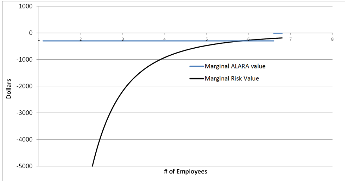
Figure 38. Comparison of Marginal Risk Value (LNT) with marginal ALARA value at a watch level of 0.5 rem/year. Staff levels are incremented by 0.1 workers. The discontinuity is due to the piece-wise definition of the ALARA value; the break occurs where the first derivative does not exist.
